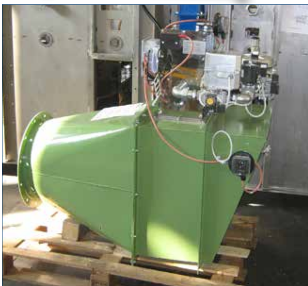
Application with VDM burner and process air duct
